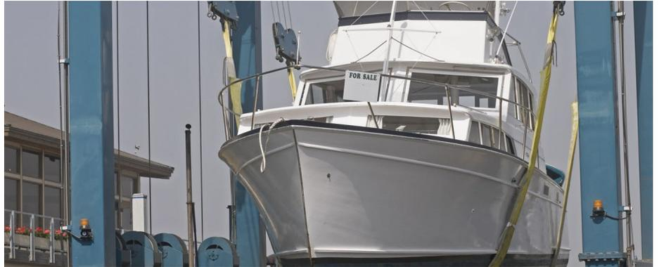
Boat hoist slings are an often overlooked yet critical component of your boat hoist system. These synthetic web slings, made of either nylon or polyester, are susceptible to many deteriorating or damaging conditions during regular use. Effective protocols for sling inspection, care, and replacement must be in place to prevent potential damage, injury, or death from sling failure.
