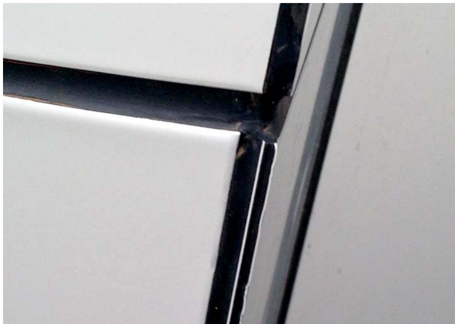
Photograph showing the PE core of Aluminium Composite Panel.
